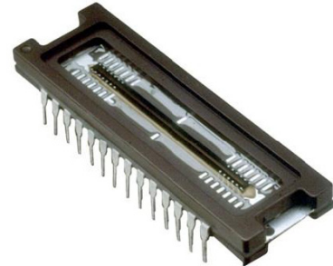
Figure 1. KLI-2113 Linear CCD Image Sensor
