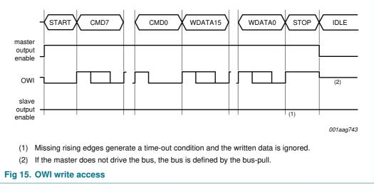
**Note**: As already mentioned in <u>Section 13.1</u>, the command mode has to be entered using the write procedure. If command mode is not entered, digital communication is not possible and the sensor operates in normal operating mode. After changing an address, the time  $t_{prog}$  must elapse before changing another address. Finally the checksum must be recalculated and written, after changing the contents of the EEPROM (see Section 13.4).
