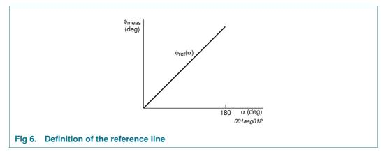
The angular range is set to  $\alpha_{max}$  = 180° and the clamping voltages are programmed to  $V_{(CL)I}$  = 5 %V<sub>DD</sub> and  $V_{(CL)u}$  = 95 %V<sub>DD</sub> for a valid definition of errors.
