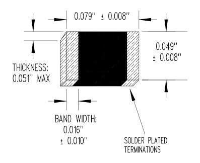
RESISTANCE @  $+25^{\circ}\text{C} = 10,000 \ \Omega \pm 5\%$ RESISTANCE/TEMPERATURE CURVE = "J" TEMPERATURE COEFFICIENT @  $+25^{\circ}\text{C} = -4.4\%$ /'C NOMINAL BETA " $\beta$ " (+25 TO  $+85^{\circ}\text{C}$ ) = 3,976°K NOMINAL MAXIMUM TEMPERATURE RATING =  $+125^{\circ}\text{C}$
