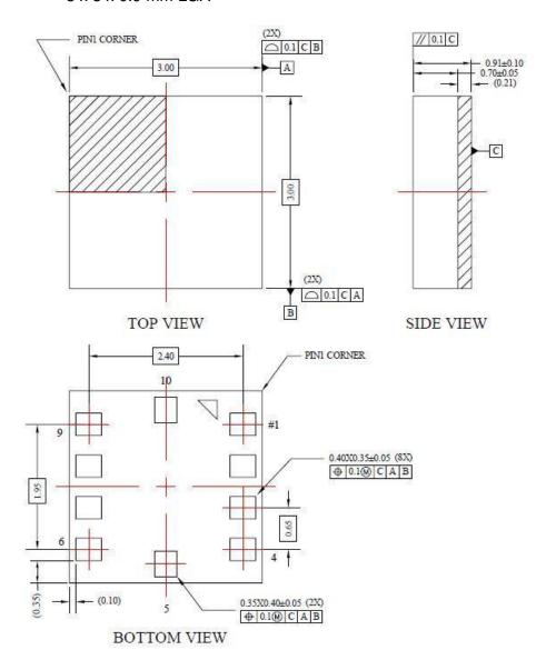
All dimensions and tolerances conform to ASME Y14.5M-1994
