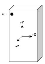
When device is accelerated in +X, +Y or +Z direction, the corresponding output will increase.
