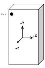
When device is accelerated in +X, +Y or +Z direction, the corresponding output will increase.
