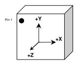
When device is accelerated in +X, +Y or +Z direction, the corresponding output will increase.
