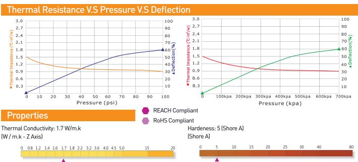
In the thermal resistance vs pressure vs deflection charts L37-3 provides low thermal impedance.
