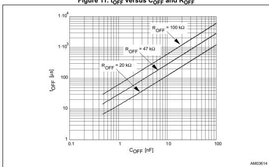
Figure 11.  $t_{OFF}$  versus  $C_{OFF}$  and  $R_{OFF}$
