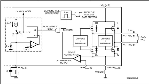
Figure 9. PWM current controller simplified schematic
