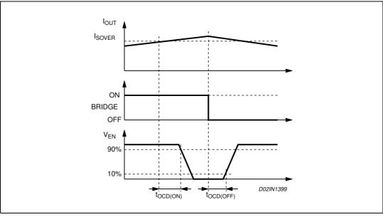
Figure 4. Overcurrent detection timing definition
