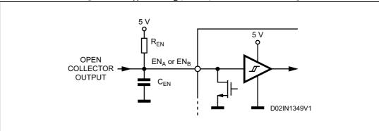
Figure 8. EN<sub>A</sub> and EN<sub>B</sub> pins push-pull driving
