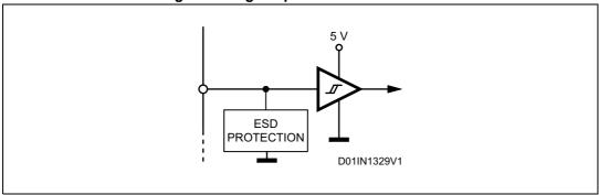
Figure 7. EN<sub>A</sub> and EN<sub>B</sub> pins open collector driving
