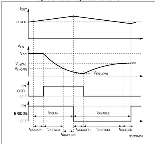
Figure 15. Overcurrent protection waveforms
