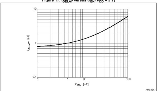
Figure 17.  $t_{DELAY}$  versus  $C_{EN}$  ( $V_{DD} = 5 V$ )
