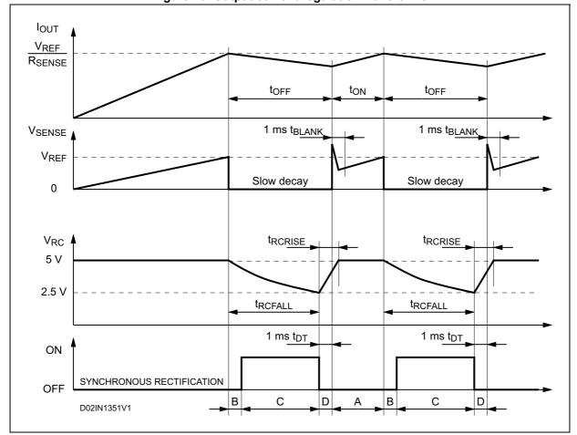
Figure 10. Output current regulation waveforms
