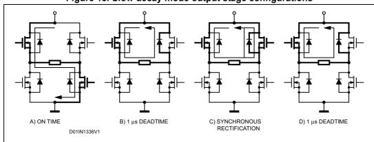
Figure 13. Slow decay mode output stage configurations
