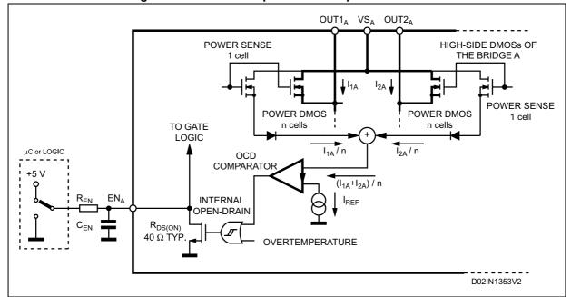
Figure 14. Overcurrent protection simplified schematic
