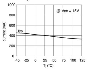
Figure 7. Output Sink Current vs. Temperature
