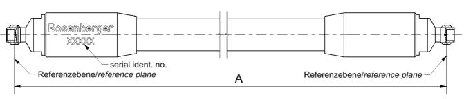
All dimensions are in mm; tolerances: ± 3mm for A ≤ 300 mm; ± 1% for A > 300 mm
