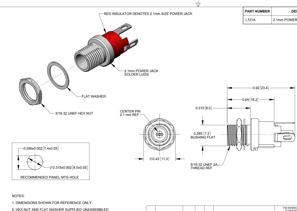
3. MATERIAL: HOUSING, HEX NUT - COPPER ALLOY, NICKEL PLATED INSULATOR HOUSING - THERMOPLASTIC, RED TERMINAL INSULATORS - PHENOLIC FLAT WASHER - STEEL, NICKEL PLATED
