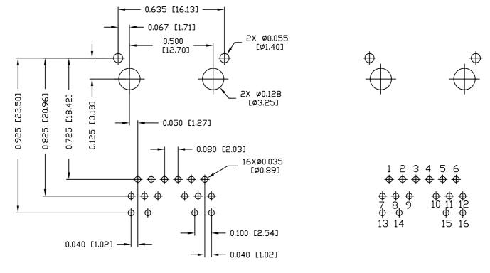
ORIGINATED BY TITLE DATE PART NO. / DRAWING NO. METRIC DIM. AS REFERENCE STANDARD DIM. 11-25-05 QIN/BILL bel L8261X1T43-F TOL. IN INCH gigabit MagJack® REV. : UNIT: INCH [mm] (8 cores, Tab Up) X. DRAWN BY DATE FILE NAME SCALE : N/A SIZE: A4 COMPONENTS ON A COMMICTED PLANET .XX L826-1X1T-43-F TING 11-25-05 L8261X1T43-FB.DWG PAGE: 4
