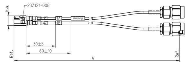
All dimensions are in mm; tolerances:  $\pm$  3mm for A  $\leq$  300 mm;  $\pm$  1% for A > 300 mm
