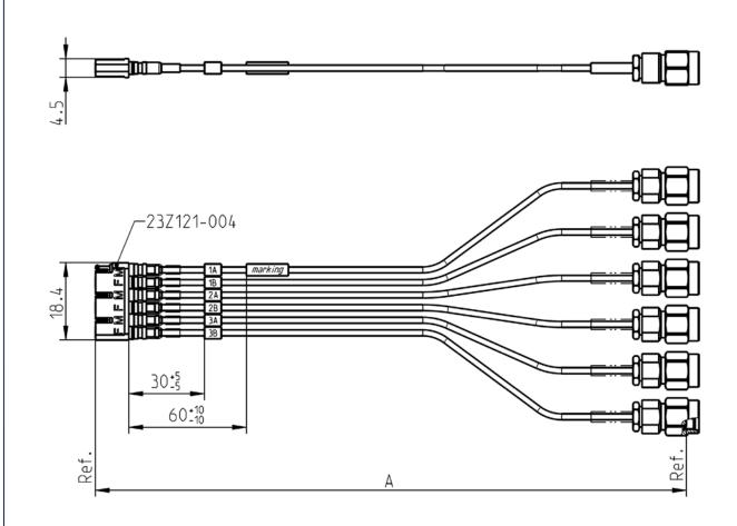
All dimensions are in mm; tolerances: ± 3mm for A ≤ 300 mm; ± 1% for A > 300 mm
