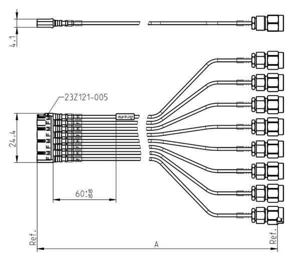
All dimensions are in mm; tolerances:  $\pm$  3mm for A  $\leq$  300 mm;  $\pm$  1% for A > 300 mm
