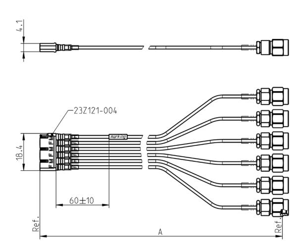
All dimensions are in mm; tolerances:  $\pm$  3mm for A  $\leq$  300 mm;  $\pm$  1% for A > 300 mm
