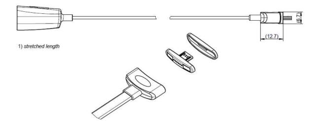
All dimensions are in mm; tolerances according to ISO 2768 c
