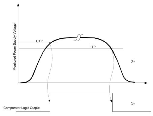
During power supply ramp-up the comparator output changes from logic 0 to 1 when the power supply voltage crosses the upper trip point (UTP). During ramp down the comparator output changes from logic state 1 to 0 when the power supply voltage crosses the lower trip point (LTP). To monitor for over voltage fault conditions, the UTP should be used.
