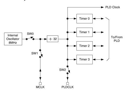
The internal oscillator runs at a fixed frequency of 8 MHz. This signal is used as a source for the PLD and timer clocks. It is also used for clocking the comparator outputs and clocking the digital filters in the voltage monitor circuits and ADC. The LA-ispPAC-POWR1014/A can be programmed to operate in three modes: Master mode,
