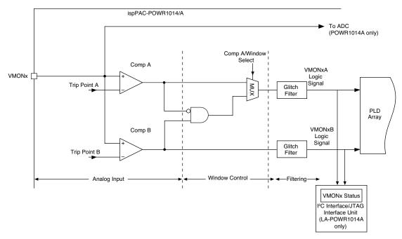
Figure 5-7 shows the functional block diagram of one of the 10 voltage monitor inputs - 'x' (where x = 1...10). Each voltage monitor can be divided into three sections: Analog Input, Window Control, and Filtering.
