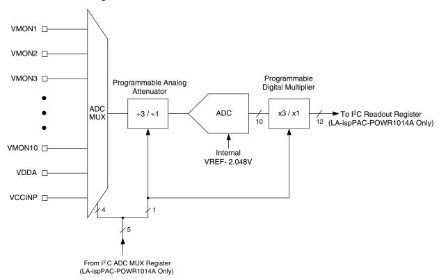
Figure 5-9 shows the ADC circuit arrangement within the LA-ispPAC-POWR1014A device. The ADC can measure all analog input voltages through the multiplexer, ADC MUX. The programmable attenuator between the ADC mux and the ADC can be configured as divided-by-3 or divided-by-1 (no attenuation). The divided-by-3 setting is used to measure voltages from 0V to 6V range and divided-by-1 setting is used to measure the voltages from 0V to 2V range.
