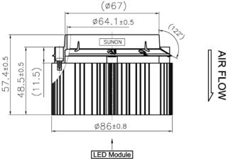
Assembly direction of customer's LED Module
