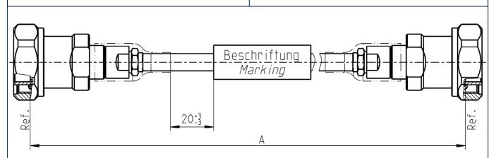
All dimensions are in mm; tolerances:  $\pm$  3mm for A  $\leq$  300 mm;  $\pm$  1% for A > 300 mm
