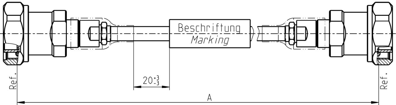
All dimensions are in mm; tolerances:  $\pm 3$  mm for  $A \leq 300$  mm;  $\pm 1\%$  for  $A > 300$  mm
