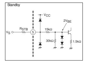
Note that the standby pin (pin 5) incorporates the anti-electrostatic diode, allowing the cu orrent to flow through the diode when the potential of  $V_{CC}$  pin 7 decreases below that of pin 5.
