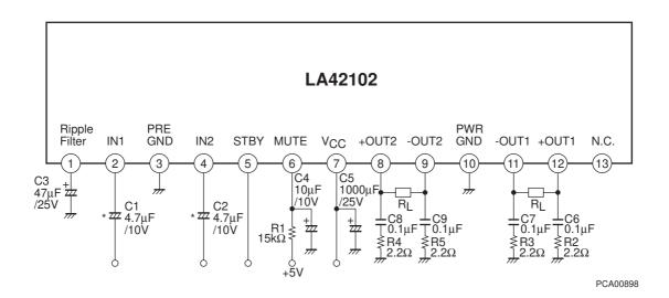
\* LA42102 employs the zero-bias type input circuit, with the input pin potential being nearly zero (about 0.01V). Accordingly, the polarity must be determined according to the DC potential of a circuit connected to the previous stage of LA42102.
