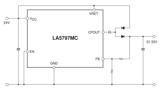
External circuit diagram ( $V_{CC} = 15V$ )
