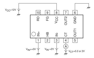
CT pin charge/discharge voltage (VCT)
