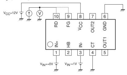
FG, RD input pin leakage current (IFGL, RDL)
