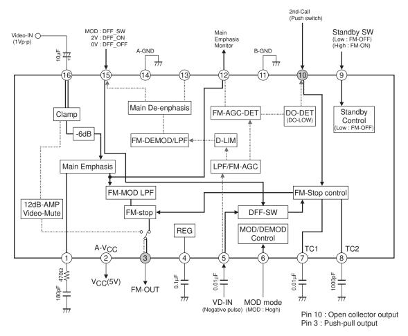
Application Circuit Example2 Demodulation (Monitor)
