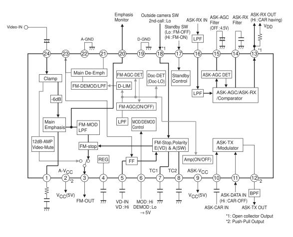
Application Circuit Example2 Demodulation (Inside monitor)
