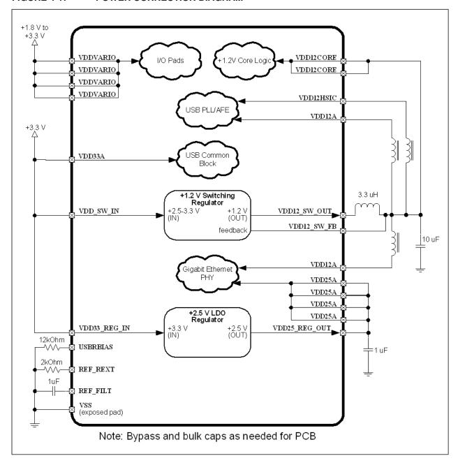
Note: For 3.3V I/O operation, the VDDVARIO and +3.3V supplies may be connected together.
