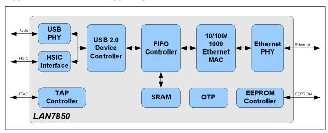
FIGURE 2-1: INTERNAL BLOCK DIAGRAM
