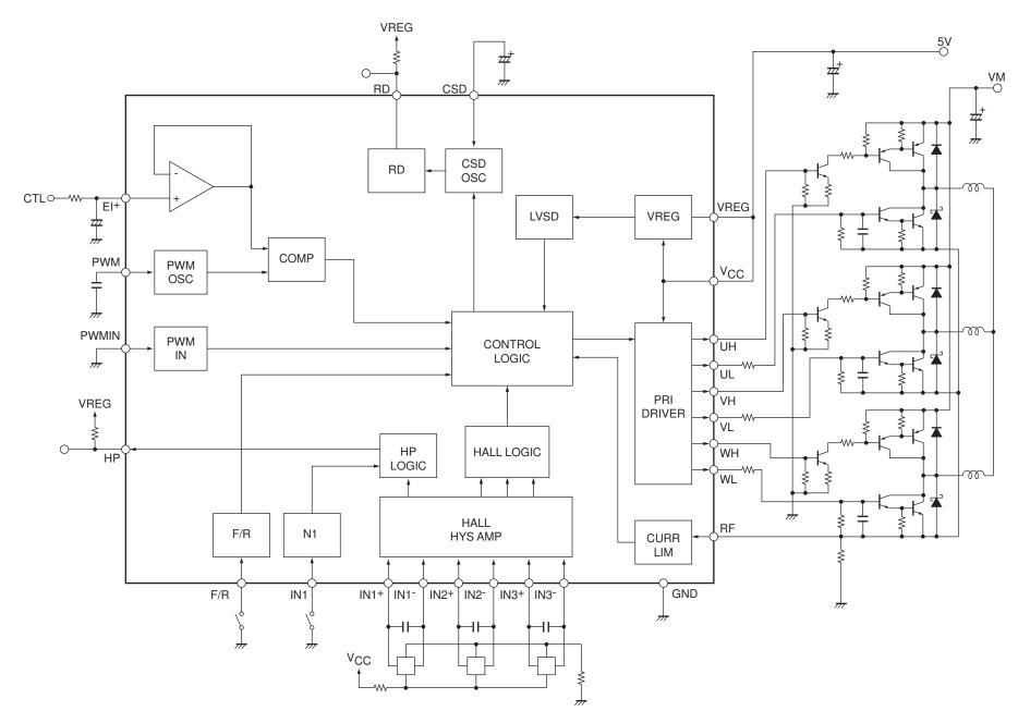
**Application Example 2**54 MOS transistor drive (low side PWM) using a 12V single-voltage power supply
