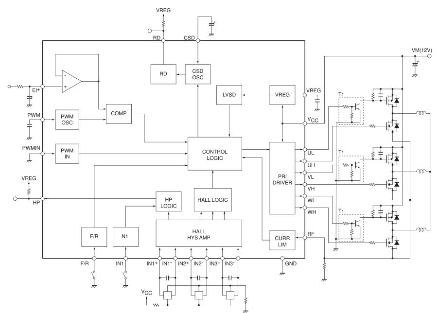
**Application Example 3**MOS transistor drive (low side PWM)
