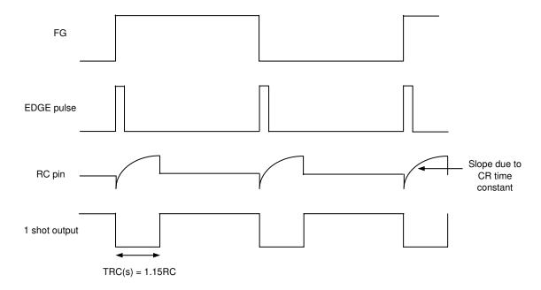
Furthermore, by changing the pulse width as determined by the CR time constant, the VCTL versus speed slope can be changed as shown in the speed control diagram of the previous section.
