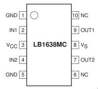
Note: both ground pins must be grounded.
