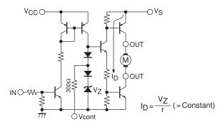
As shown in the left diagram, the Vcont pin outputs the voltage of the band gap Zener VZ +VF (= 1.93V).
