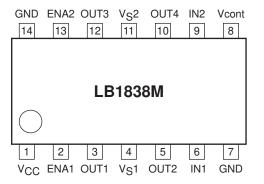
Note: Both GND pins should be connected to ground.
