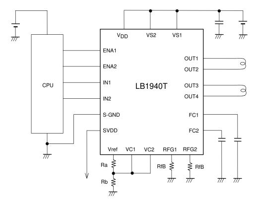
At constant-current control: The OUT current is controlled so that the RFG pin voltage is equal to the VC input pin voltage.
