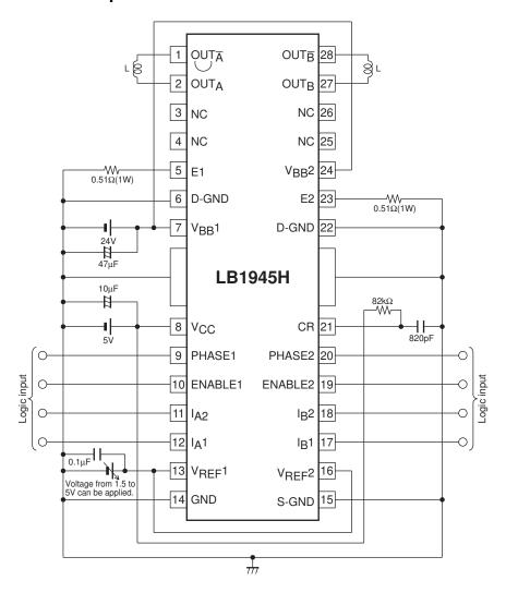
The fin on the bottom of HSOP-28H package and the fins between pins 7 and 8 and 21 and 22 should be grounded.
