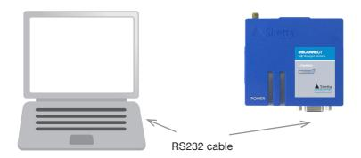
The USB-Serial converter will appear in windows Device Manager as 'Prolifc USB to serial' and will be allocated a COM port number.
