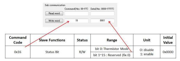
Press [Write Word] to enable Thermistor
