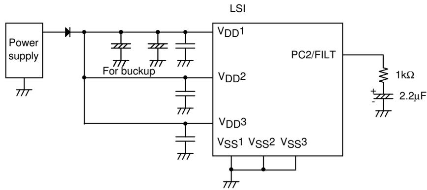
Example 2: When data is being backed up in the HOLD mode, the H level output at any ports is not sustained and is unpredictable.
