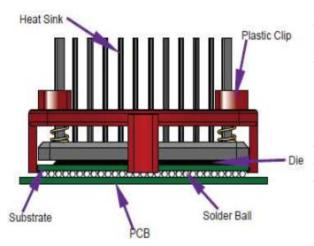
Wakefield-Vette's heat sink assembles onto chip set using the space that is between the PCB and the substrate of the solder balls. The solder balls provide a minimal gap of .5mm to .7mm. Attachment feature is below a .4mm thickness. The clipping system will not interfere or damage chip. Contact area is the edge of chip.
