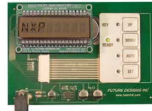
Typical SBC Application for Keypad Tester
