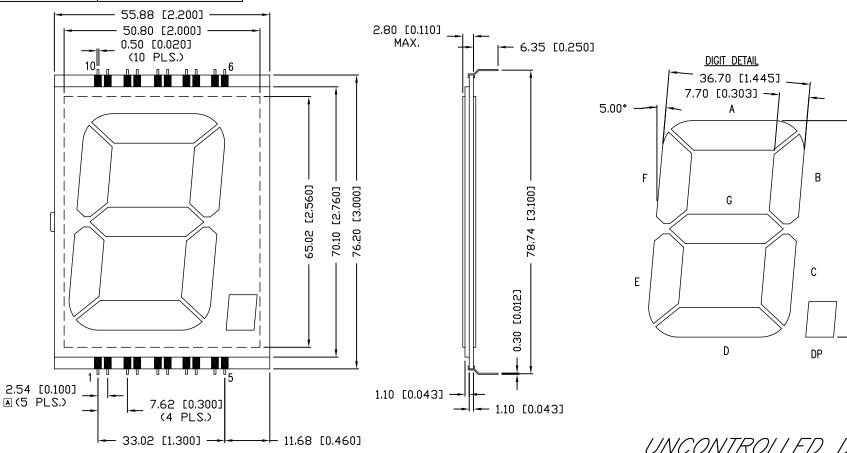
\*UNLESS OTHERWISE SPECIFIED TOLERANCES PER DECIMAL PRECISION ARE: X=±1 (±0.039), X.XX=±0.5 (±0.020), X.XXX=±0.25 (±0.010), X.XXX=±0.127 (±0.005). LEAD SIZE=±0.05 (±0.002), LEAD LENGTH=±0.75 (±0.030). MIN= +DECIMAL PRECISION
