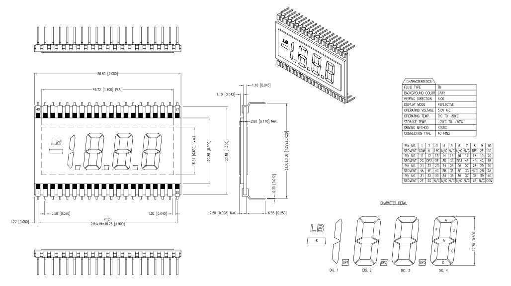
\*UNLESS OTHERWISE SPECIFIED TOLERANCES PER DECIMAL PRECISION ARE: X=±1 (±0.039), X.X=±0.5 (±0.029), X.XX=±0.25 (±0.010), X.XXX=±0.127 (±0.005). LEAD SIZE=±0.05 (±0.002), LEAD LENGTH=±0.75 (±0.030). MIN= +DECIMAL PRECISION MAX.= +0.00 (±0.001), MIN= +DE
