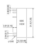
NOTE: Pin tolerance ±0.05mm
