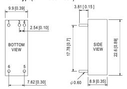
NOTE: Pin tolerance ±0.05mm
