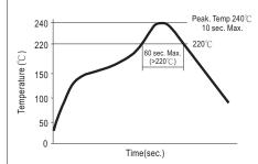
Remark : The curve applies only to the "Hot Air Reflow Soldering"
