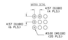
\*UNLESS OTHERWISE SPECIFIED TOLERANCES PER DECIMAL PRECISION ARE: X=±1 (±0.039), X.X=±0.5 (±0.020), X.XX=±0.5 (±0.010), X.XXX=±0.127 (±0.005). LEAD SIZE=±0.05 (±0.002), LEAD LENGTH=±0.75 (±0.030). MIN= +DECIMAL PRECISION MAX.= +0.00 -DECIMAL PRECIS
