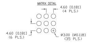
\*UNLESS OTHERWISE SPECIFIED TOLERANCES PER DECIMAL PRECISION ARE: X=±1 (±0.039), X.X=±0.5 (±0.020), X.XX=±0.25 (±0.010), X.XXX=±0.127 (±0.005). LEAD SIZE=±0.05 (±0.002), LEAD LENGTH=±0.75 (±0.030). MIN= +DECIMAL PRECISION -0.000
