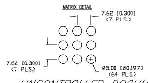
\*UNIESS OTHERWISE SPECFED TOLERANCES PER DECIMAL PRECISION ARE: X=±1 (±0.039), XX=±0.5 (±0.020), XXX=±0.25 (±0.010), XXXX=±0.127 (±0.005). LEAD 97ZE=±0.05 (±0.002), LEAD LENGTH=±0.75 (±0.030). NN= +0ECIMAL PRECISION MAX.= +0.00 (±0.000), XXXX=±0.127 (±0.005).
