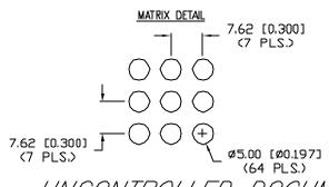
\*UNLESS OTHERWISE SPECIFED TOLERANCES PER DECIMAL PRECISION ARE: X=±1 (±0.039), XX=±0.5 (±0.020), XXX=±0.25 (±0.010), XXXX=±0.127 (±0.005). LEAD SIZE=±0.05 (±0.002), LEAD LENGTH=±0.75 (±0.030). NN= +DECIMAL PRECISION MAX.= +DECIMAL PRECISION MAX.
