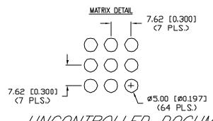
\*UNIESS OTHERWISE SPECFED TOLERANCES PER DECIMAL PRECISION ARE: X=±1 (±0.039), XX=±0.5 (±0.020), XXX=±0.25 (±0.010), XXXX=±0.127 (±0.005). LEAD 97ZE=±0.05 (±0.002), LEAD LENGTH=±0.75 (±0.030). NN= +0ECIMAL PRECISION MAX.= +0.00 (±0.000), XXXX=±0.127 (±0.005).
