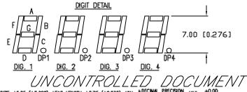
\*UNILESS OTHERWISE SPECIFIED TOLERANCES PER DECIMAL PRECISION ARE: X=±1 (±0.039), XX=±0.5 (±0.020), XXX=±0.25 (±0.010), XXXX=±0.127 (±0.005). LEAD SIZE=±0.05 (±0.002), LEAD LENGTH=±0.75 (±0.030). MN= +DECIMAL PRECISION ARE: X=±1 (±0.039), XX=±0.5 (±0.020), XXX=±0.25 (±0.010), XXXX=±0.127 (±0.005).
