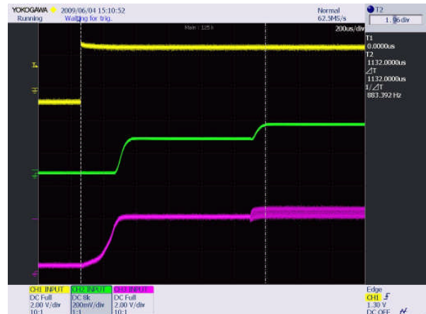
V_{IN} = 3.6\text{ V} , Ch1 – PWM, Ch2 – LED current (400 mA/div), Ch3 – Output voltage
